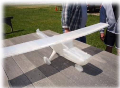
Above: (lft.) Yes...that's a 3D Printed Airplane!! The project was a collaboration between Bill Alexander and Rich Cansler utilizing software by 3D Lab Print. The intricate design took somewhere between 150—200 hours print and involved about $15-$18 worth of material.. (cntr.) Jerry Brown demonstrated his Convergence VOL...lands and takes off like a typical multi-rotor drone, but flies like an airplane. (rt.) "Chef" Bill Alexander doing his thing. Once the grilling was underway, everyone's attention turned to "food!"
