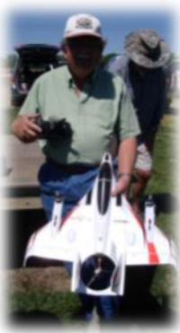
Above: (lft.) Yes...that's a 3D Printed Airplane!! The project was a collaboration between Bill Alexander and Rich Cansler utilizing software by 3D Lab Print. The intricate design took somewhere between 150—200 hours print and involved about $15-$18 worth of material.. (cntr.) Jerry Brown demonstrated his Convergence VOL...lands and takes off like a typical multi-rotor drone, but flies like an airplane. (rt.) "Chef" Bill Alexander doing his thing. Once the grilling was underway, everyone's attention turned to "food!"
