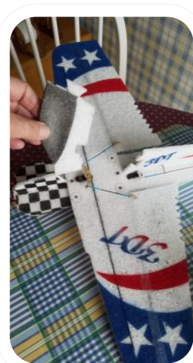
The Cockpit/Canopy section of the fuselage is held in place by magnets and an indexing tab. It’s removable to allow access to the wing-mounting screws and for separating the wing from the fuselage.
